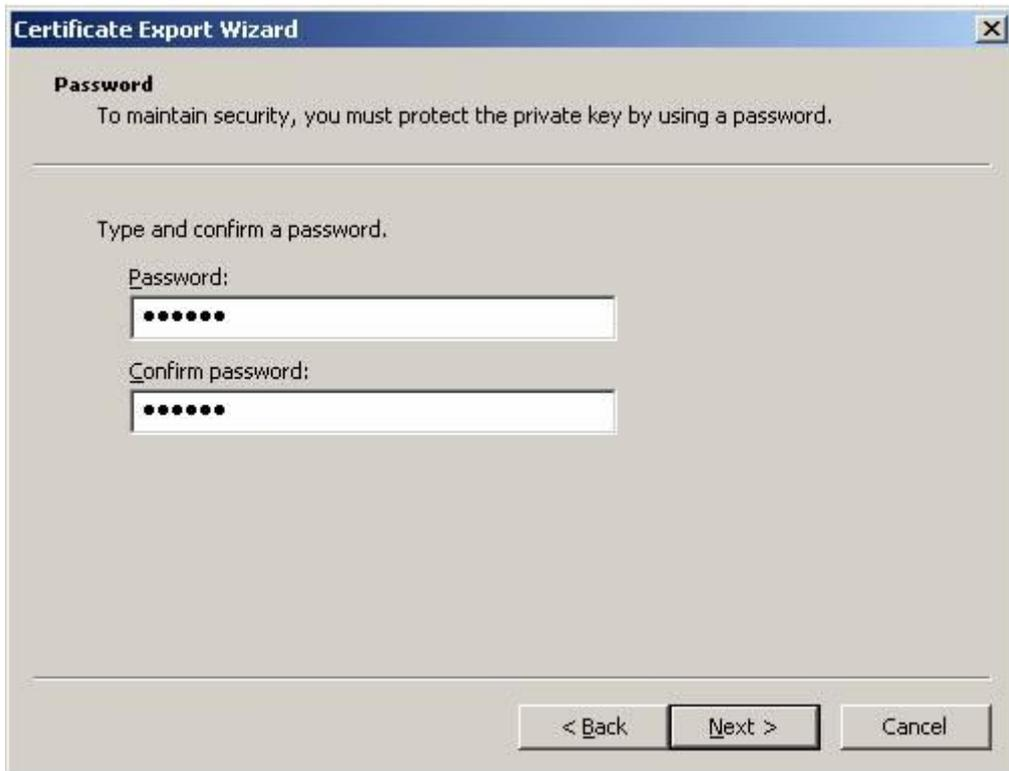
**Figure 3.21:** Enter a password in order to protect the private key
