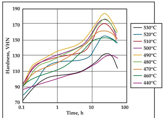
Fig. 4 — Hardness-time curves for Al alloy 380 solution treated at different temperatures for 15 minutes and aged at a temperature of 150°C.
