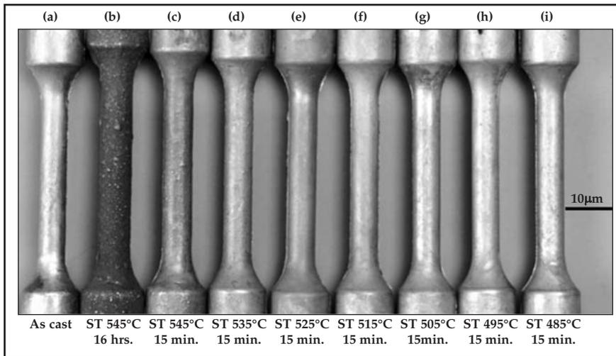
Fig. 1 — Surface appearance of Al alloy 360 HPDC tensile specimens in the as-cast condition and after different solution treatment schedules.
