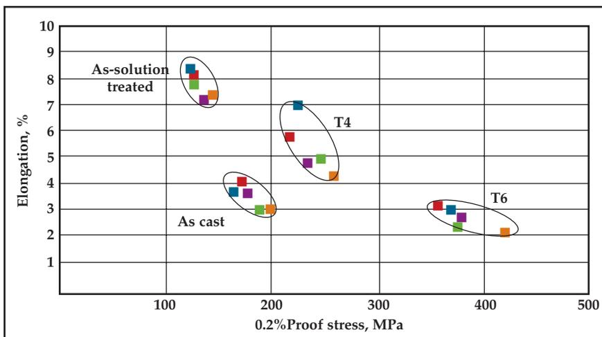
Fig. 5 — Properties of the alloys shown in Table 4 comparing the 0.2% proof stress and elongation for the as-cast, as solution treated, T4, and T6 conditions.
