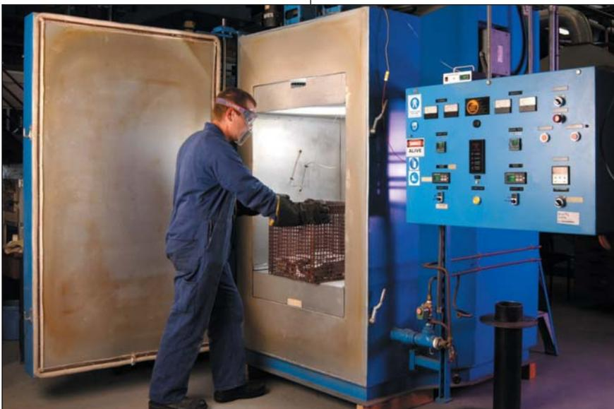
Aluminum diecast samples being loaded into furnace for heat treating
