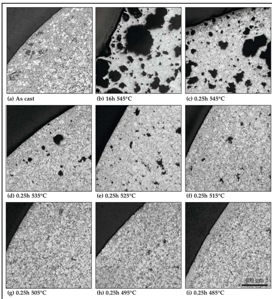
Fig. 2 — Microstructures of the Al 360 alloy in the different heat treated conditions shown in Fig. 1. Etchant: 0.5% HF.
