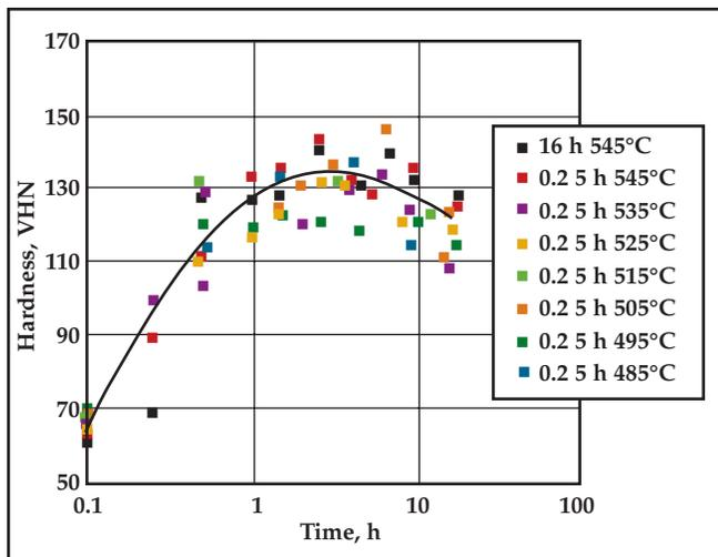
Fig. 3 — Hardness-time curves for Al alloy 360 aged at a temperature of 180°C following solution treatment at different times and temperatures.
